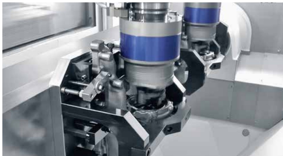
KOMET KomTronic® U-axes during V-band machining with two spindles
