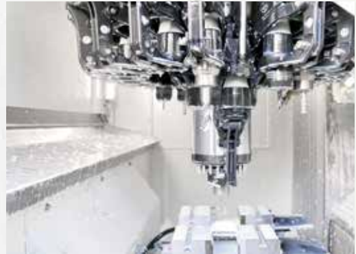
The core component of the FZ15 W baseline: The basket tool changer, with a changeover time of 2.1 seconds for maximum productivity
